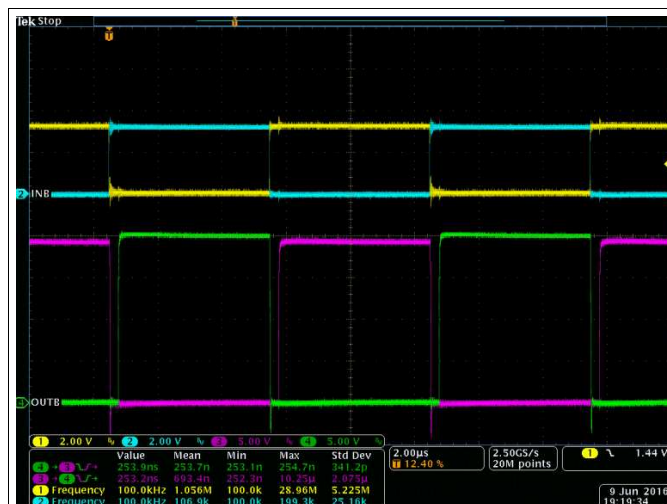
Figure 45. Bench Test Waveform for INA/B and OUTA/B
