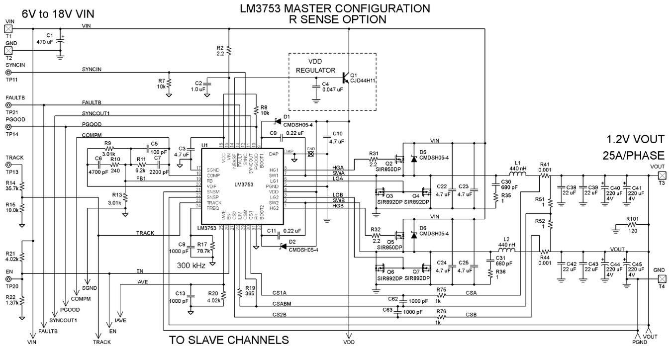
Figure 34. Master with Resistor Sense
