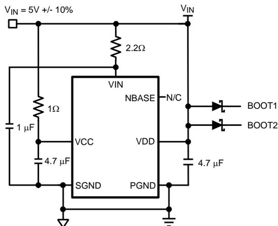
Figure 14. Power Connections for  $V_{IN} = 5V$
