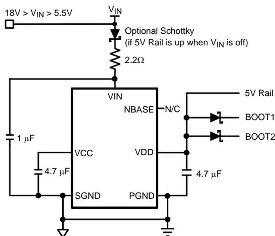
Figure 13. Power Connections Using a System 5V Rail
