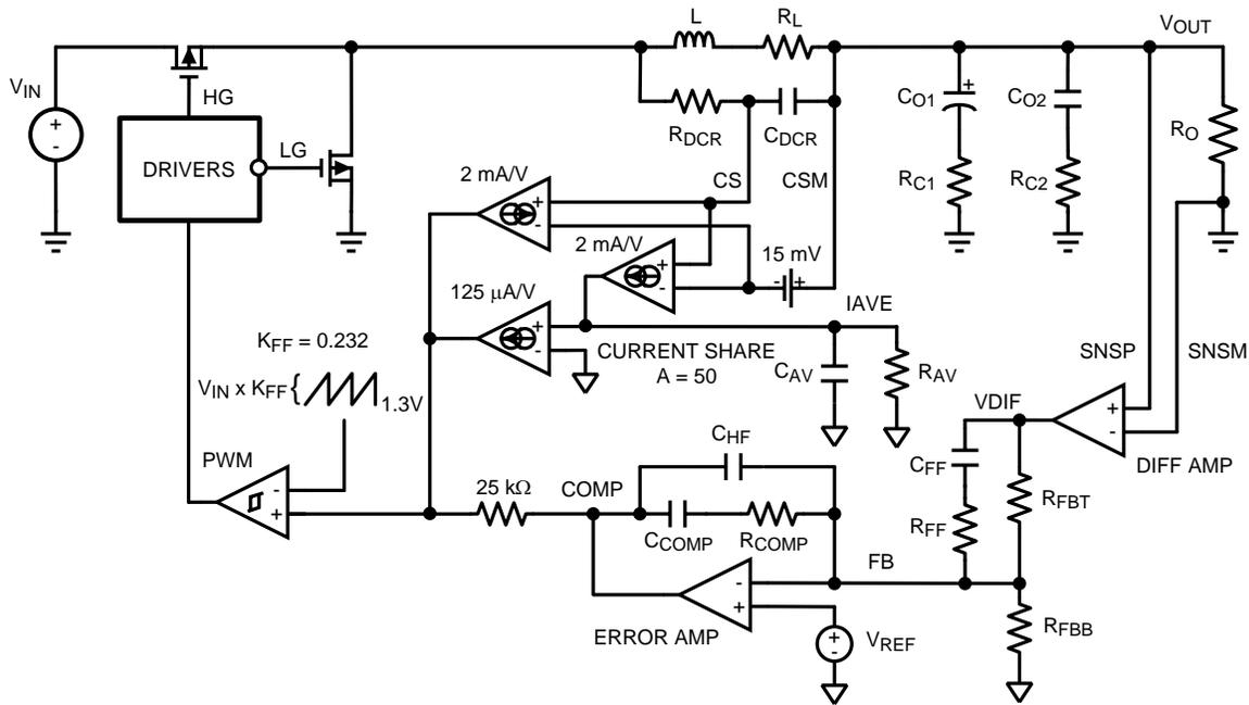
Figure 24. Power Stage, Error Amplifier and Current Sharing
