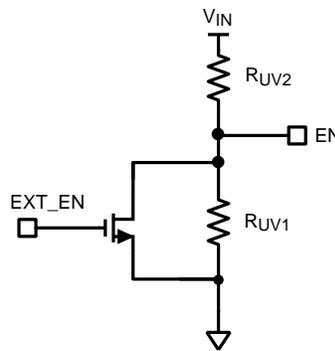
**Figure 15. Input Voltage UVLO with External Enable**
