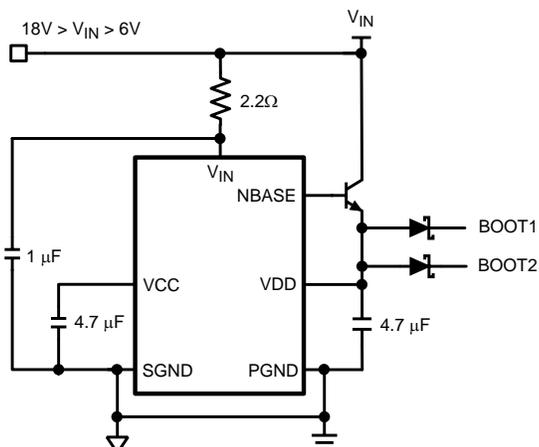
Figure 12. Power Connections Using the Internal Regulator
