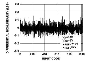
FIGURE 1. DIFFERENTIAL NONLINEARITY vs CODE
