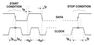
START, STOP & TIMING DETAILS OF I<sup>2</sup>C INTERFACE
