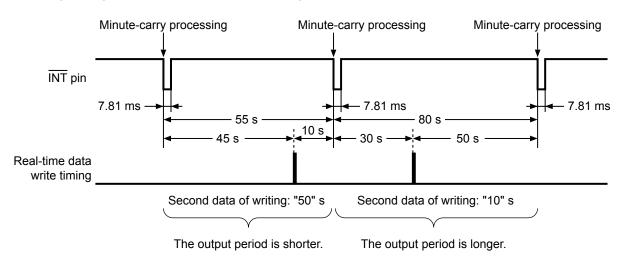
Figure 32 Timing of Minute-periodical Interrupt Output 2
