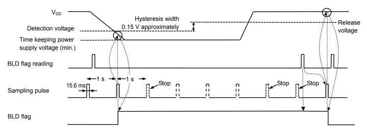
Figure 25 Timing of Low Power Supply Voltage Detection Circuit
