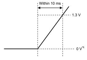
\*1. 0 V indicates that there are no potential differences between the VDD pin and VSS pin of the S-35190A.
