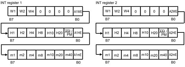
Figure 17 INT Register 1 and INT Register 2 (Alarm-Time Data)
