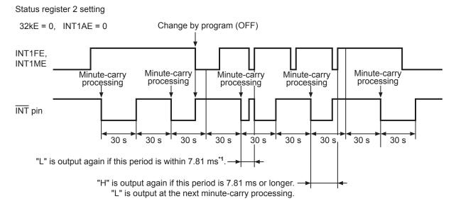
\*1. Setting the output mode disable makes the pin output "H", while the output from the  $\overline{\text{INT}}$  pin is in "L". Note that pin output is set to "L" by setting the output mode enable again.
