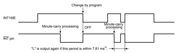
\*1. Pin output is set to "H" by disabling the output mode within 7.81 ms, because the signal of this procedure is maintained for 7.81 ms. Note that pin output is set to "L" by setting the output mode enable again.
