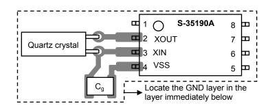
Figure 46 Connection Diagram 2
