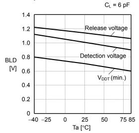
13. BLD detection, release voltage, V<sub>DDT</sub> (min.) vs. Temperature characteristics
