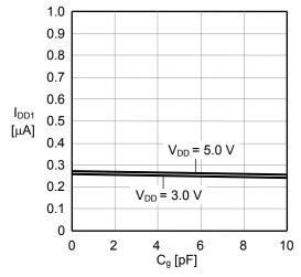
2. Current consumption when 32.768 kHz is output vs.  $V_{\text{DD}}$  characteristics
