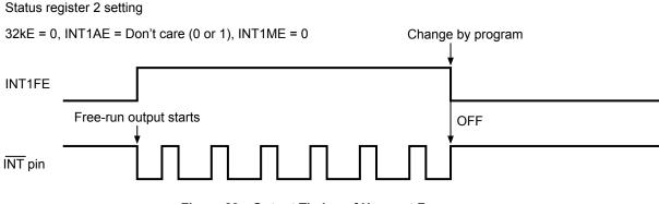
Figure 29 Output Timing of User-set Frequency
