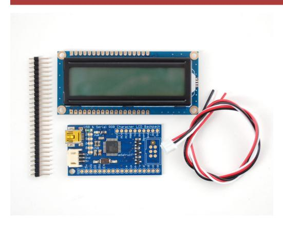
The backpack comes with a piece of header you can use to fit the display on. Its handy to have a solderless breadboard to attach the header on straight.
