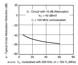
Fig. 3 - Typ. Cross Modulation Distortion vs. Frequency f<sub>2</sub>
