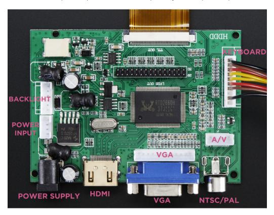
The VGA, Power and A/V inputs, the white JST ports are good alternatives to the main inputs if you don't want bulky cables coming out the sides of your driver board.
