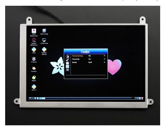
$\textbf{Power Saving -} 10s \ to \ 60s - how \ long \ it \ takes \ for \ the \ screen \ to \ shut \ off$
