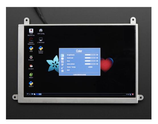
Brightness - Adjust the brightness Contrast - Adjust the contrast Hue - Adjust the hue Saturation - Adjust the saturation Color Temp - 9300K, 6500K, User
