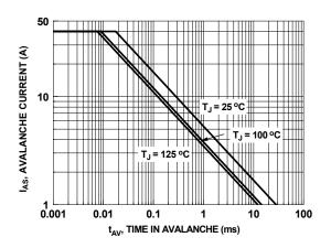
Figure 9. Unclamped Inductive Switching Capability
