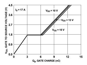
Figure 7. Gate Charge Characteristics
