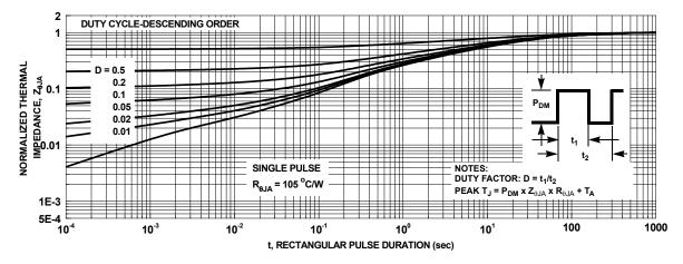
Figure 13. Junction-to-Ambient Transient Thermal Response Curve
