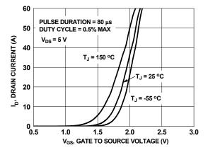
Figure 5. Transfer Characteristics
