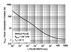
Figure 12. Single Pulse Maximum Power Dissipation
