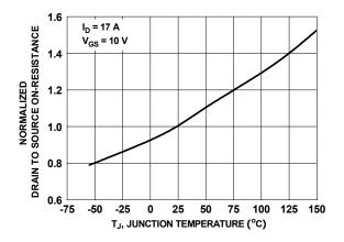
Figure 3. Normalized On Resistance vs Junction Temperature
