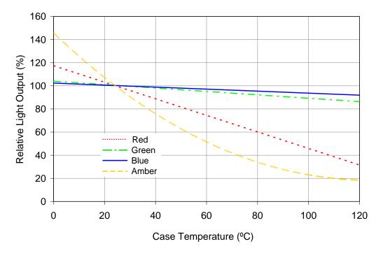
Figure 9: Typical relative light output vs. case temperature.
