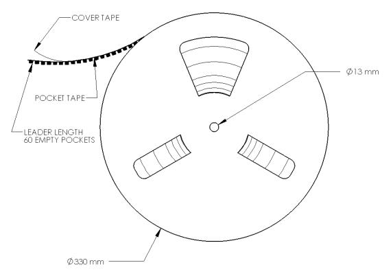
Figure 13: Emitter reel specifications (mm).
