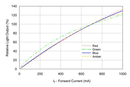
Figure 8: Typical relative light output vs. forward current @  $T_c = 25^{\circ}C$ .
