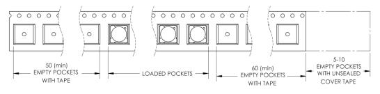
Figure 12: Emitter carrier tape specifications (mm).
