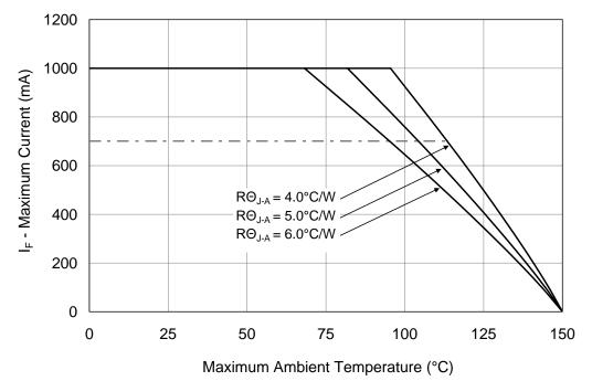
Figure 11: Maximum forward current vs. ambient temperature based on  $T_{J(MAX)}$  = 150°C.
