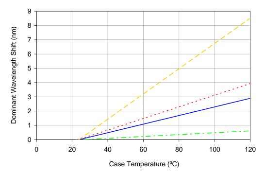
Figure 7: Typical dominant wavelength shift vs. case temperature.
