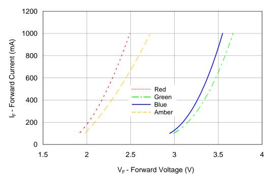
Figure 10: Typical forward current vs. forward voltage @  $T_C = 25^{\circ}C$ .
