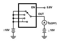
FIGURE 2. ID(OFF) TEST CIRCUIT (NOTE 8)
