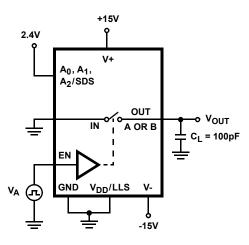
FIGURE 8A. MEASUREMENT POINTS
