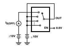
FIGURE 3. IS(OFF) TEST CIRCUIT (NOTE 8)
