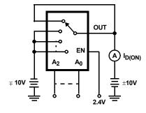
FIGURE 4. I<sub>D(ON)</sub> TEST CIRCUIT (NOTE 8)
