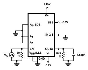
FIGURE 7A. MEASUREMENT POINTS
