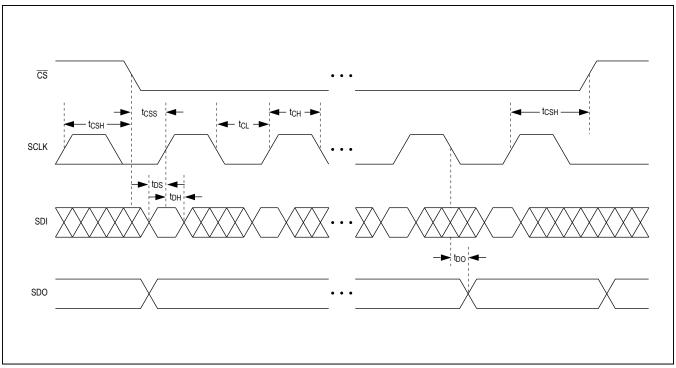
Figure 5. SPI Timing Diagram
