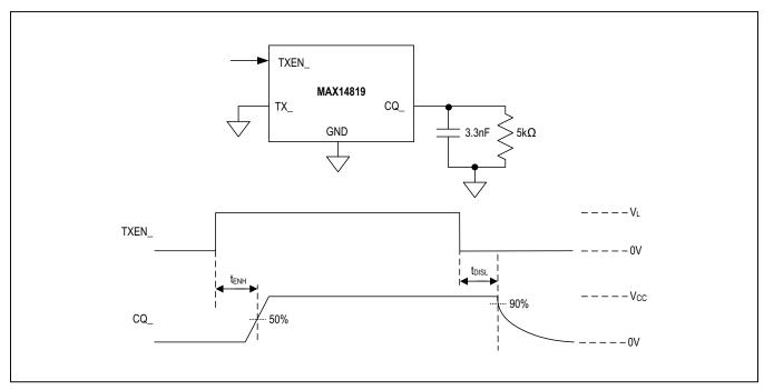
Figure 3. C/Q Driver Enable High and Disable Low Timing (INVCQ\_ = 0)
