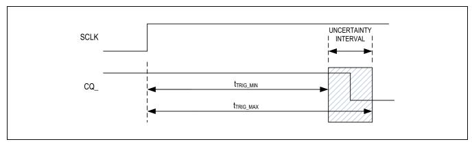
Figure 13. Trigger Delay
