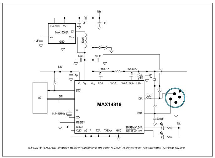
Figure 20. Using an External 5V Step-Down Regulator
