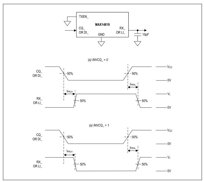
Figure 4. C/Q Receiver Propagation Delays
