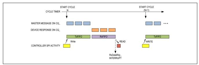
Figure 19. IO-Link Cycle Timing
