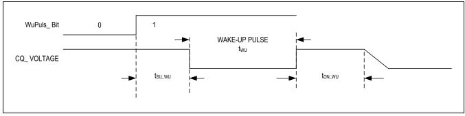
Figure 9. Wake-Up Timing
