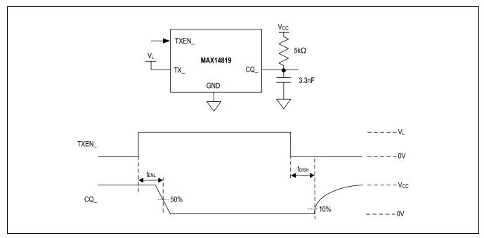
Figure 2. C/Q Driver Enable Low and Disable High Timing with External Pullup Resistor (INVCQ\_ = 0)
