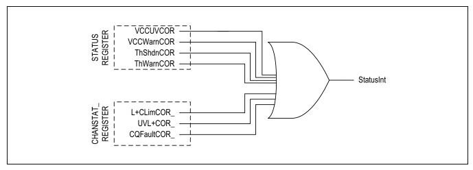
Figure 16. StatusInt Interrupt Triggers
