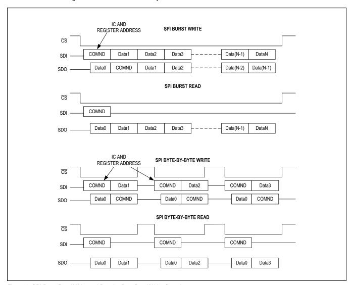
Figure 8. SPI Burst Read/Write and Byte-by-Byte Read/Write Overview
