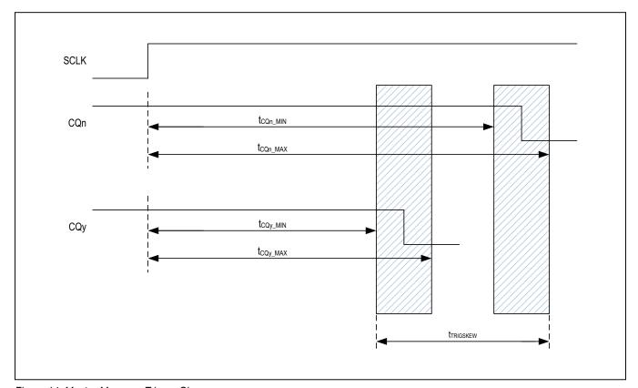
Figure 14. Master-Message Trigger Skew
