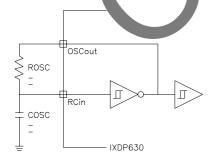
Fig. 3: IXDP630 internal Schmitt Trigger inverter oscillator ( $R_{\rm osc}$ ,  $C_{\rm osc}$  are external)
