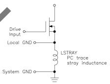
Fig. 6. Power circuit noise generation
