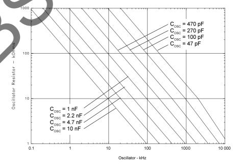
Fig. 4. Oscillator frequency component selection for IXDP630.
