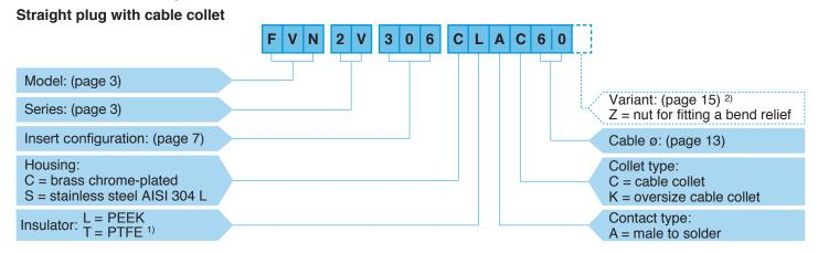
**FVN.2V.306.CLAC60** = straight plug with cable collet, 2V series, multipole type with 6 contacts, outer shell in chrome-plated brass, PEEK insulator, male solder contacts, C type collet for 6 mm diameter cable.
