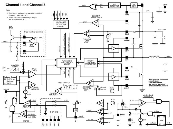
Figure 2. Channel 1 and Channel 3 Block Diagram
