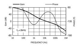
Figure 40. Higher Low Frequency Gain
