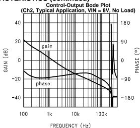
(Ch1, Typical Application, VIN = 8V, VOUT1 = 1.6V, No Load, Compensation: C14 = 390pF, R9 = 100k, C15 = 150pF, R10 = 8.2k) **Figure 24.**
