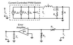
Figure 33. Small Signal Model of Buck Regulators
