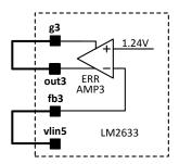
Figure 46. When Ch.3 is Not in Use
