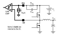
Figure 27. Current Limit Method
