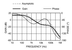
Figure 35. Example Control-Output Transfer Function Bode Plot
