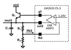
Figure 45. Channel 3 Controlling an LDO
