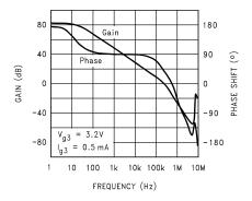
Figure 47. V<sub>FB3</sub>-to-V<sub>G3</sub> Transfer Function (theoretical)
