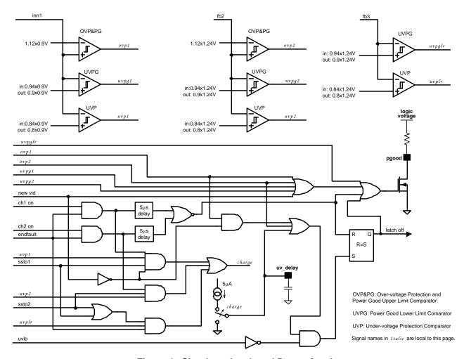
Figure 4. Shutdown Latch and Power Good
