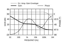
Figure 38. Example Compensation Transfer Function
