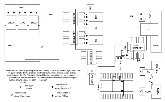
Figure 48. PCB Layout Example
