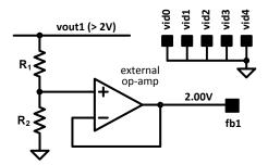
Figure 44. How to Make V<sub>OUT1</sub> Higher Than 2V
