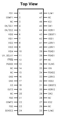
Figure 1. 48-Lead TSSOP Package See Package Number DGG0048A
