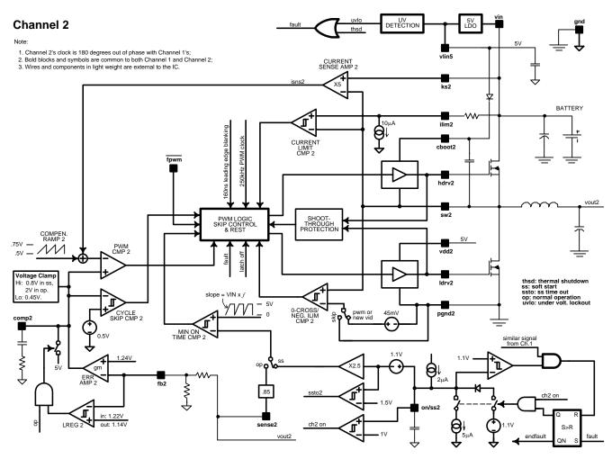
Figure 3. Channel 2 Block Diagram
