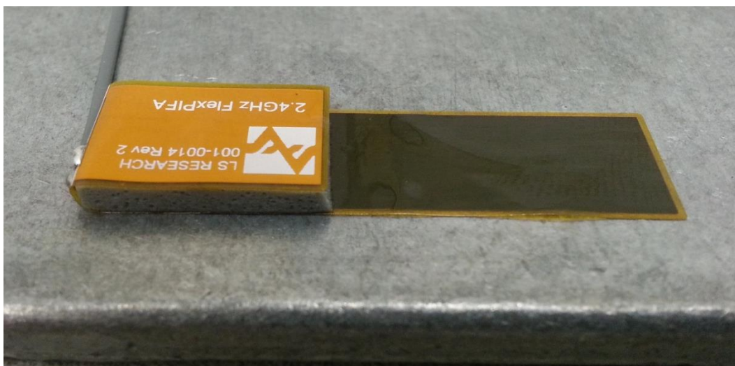
Figure 24 FlexPIFA Mounted on Metal
