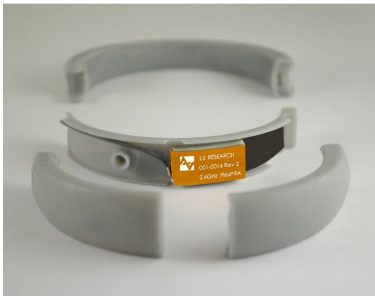
Figure 27 FlexPIFA Integrated into Bracelet
