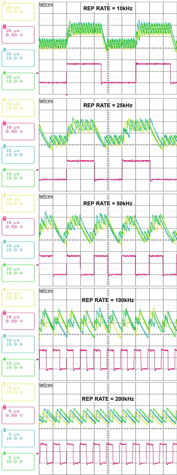
FIGURE 19. CURRENT BALANCING DURING DYNAMIC OPERATION.
