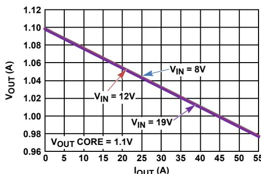
FIGURE 2. V<sub>OUT</sub> vs LOAD
