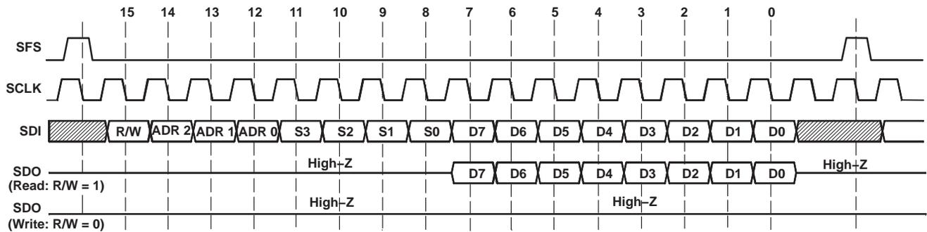
**serial command bit assignments**
