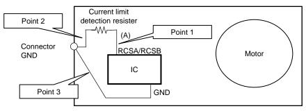
9) A high current flows into this LSI. Therefore, the common impedance of the PCB pattern cannot be ignored. Take the following points into consideration and design the PCB pattern of the motor.
