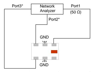
\*Impedance for ports 2 and  $3=\frac{1}{2}$  (Balanced impedance)
