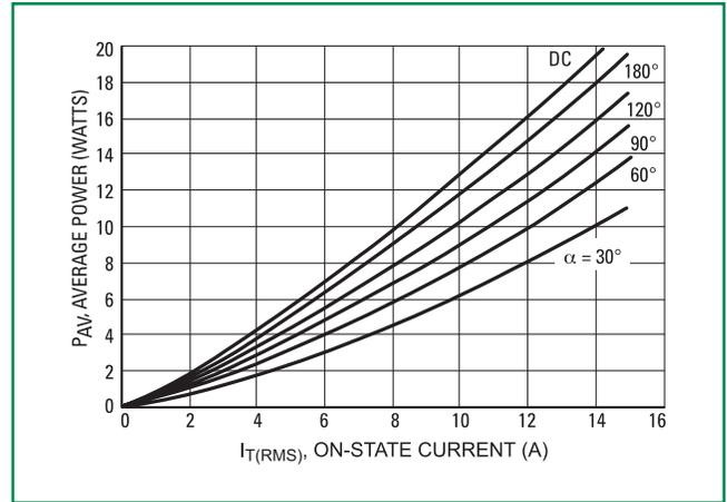
**Figure 3. On-State Characteristics**
