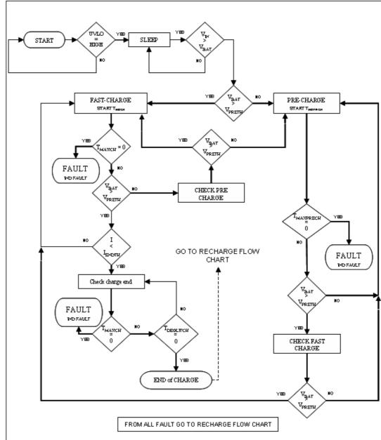
Figure 9. Charging process flow chart
