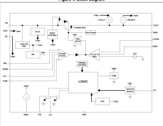
Figure 4. Block diagram
