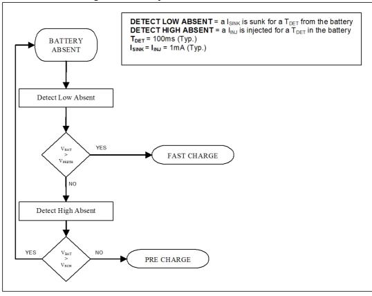
Figure 20. Battery absence detection flow chart
