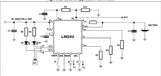
Figure 22. L6924U application schematic
