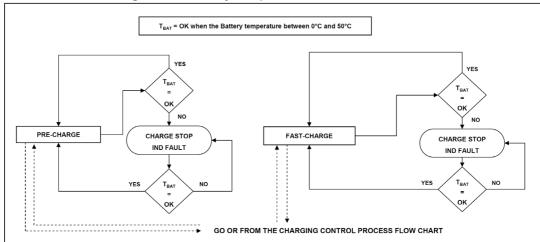
Figure 17. Battery temperature control flow chart
