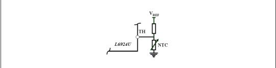
When the TH pin voltage rises and exceeds the  $V_{MINTH}$  = 50 % of  $V_{REF}$  (900 mV typ), the L6924U stops the charge, and indicates a fault by the status pins. The device re-starts to charge the battery, only when the voltage at the TH pin goes under  $V_{MINTH\_HYS}$  = 780 mV (typ).
