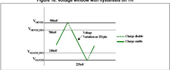
Figure 18. Voltage window with hysteresis on TH
