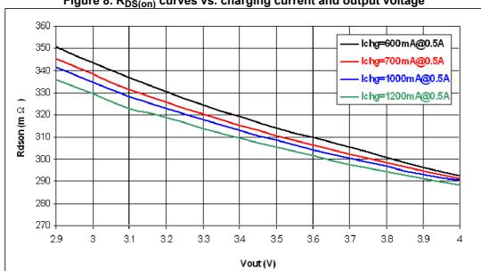
Figure 8. R<sub>DS(on)</sub> curves vs. charging current and output voltage
