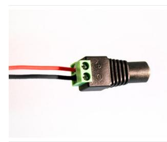
The female DC power adapter (http://adafru.it/368) mates with either of the above power supplies. Screw terminals clamp down on power wires at the end of a strip.
