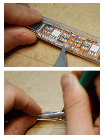
Pull off the thin rubber piece between the cuts:
