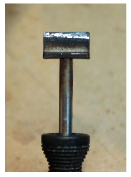
Using an X-acto knife, cut two slices from the top on either side of the solder connection:
