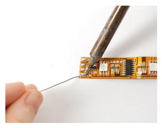
Start by soldering a red wire to the +5V power line:
