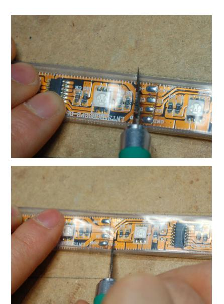
Then slice the rubber coating between the two cuts you made:
