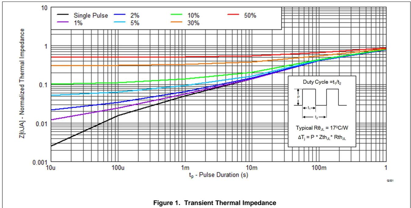
Figure 1. Transient Thermal Impedance
