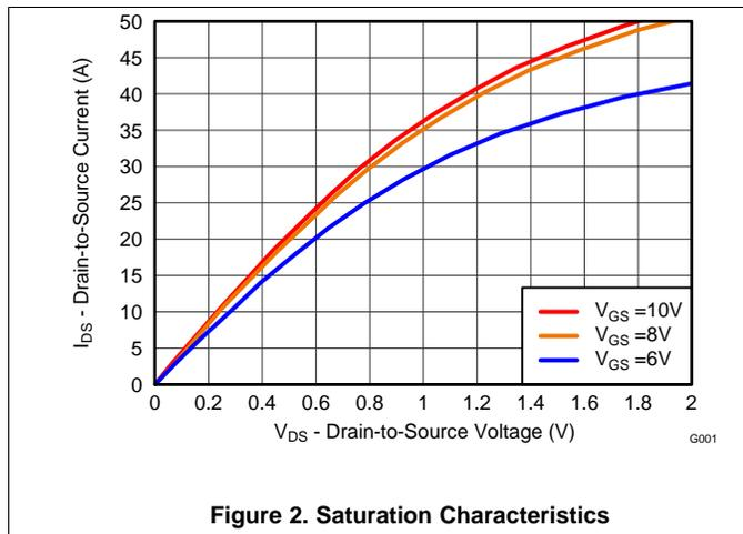
Figure 2. Saturation Characteristics
