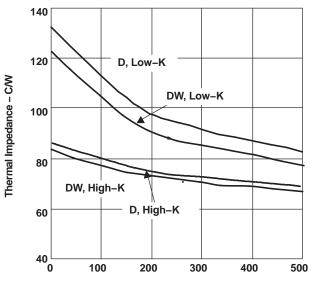
Figure 10. Thermal Impedance vs Air Flow
