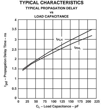
NOTE: This graph is included as an aid to the system designers. Total circuit delay varies with load capacitance. The total delay is the sum of the delay due to external capacitance and the intrinsic delay of the device. Intrinsic delay is listed in the table above as the 0 pF load condition. The incremental increase in delay between the 0 pF load condition and the actual total load capacitance represents the extrinsic, or external delay contributed by the load. Figure 5.
