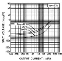
Fig.1 Input voltage vs. output current (ON characteristics)
