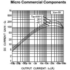
Fig.3 DC current gain vs. output current
