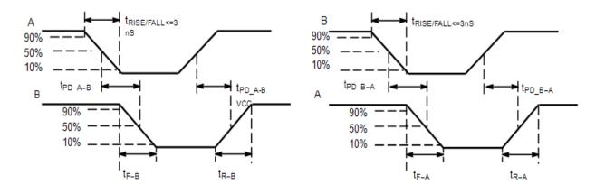
Figure 6. Definition of Timing Specification Parameters
