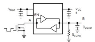
Figure 4. Open-Drain Driving A
