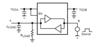
Figure 2.Rail-to-Rail Driving A
