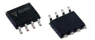
The AORN series features a narrow body (0.150") small outline SMT package. The network is constructed with a tantalum nitride resistor film on a high purity alumina substrate for improved ESD and moisture protection.
