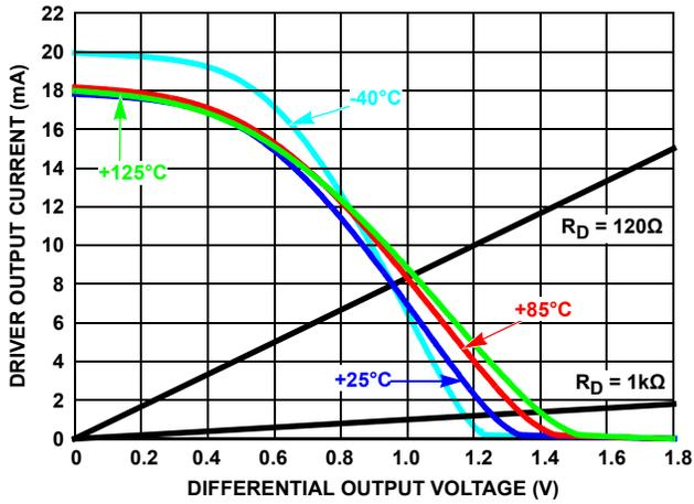
FIGURE 7. DRIVER OUTPUT CURRENT vs DIFFERENTIAL OUTPUT VOLTAGE
