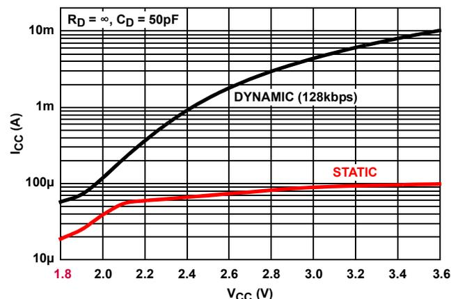
FIGURE 1. ISL32613E WITH V<sub>CC</sub> = 1.8V REDUCES OPERATING I<sub>CC</sub> BY A FACTOR OF 177 COMPARED WITH I<sub>CC</sub> AT V<sub>CC</sub> = 3.6V
