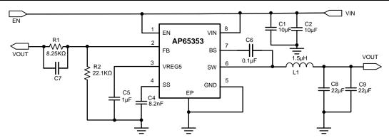
Figure 3 Typical Application of AP65353 Evaluation Board
