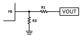
Figure 5 Feedback Divider Network
