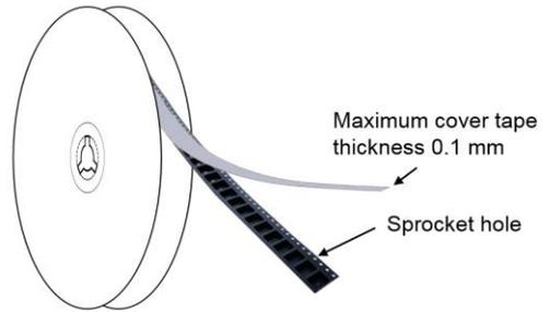
**Figure 14: Reel dimensions (mm)**
