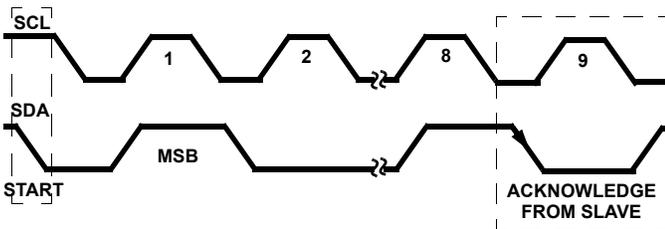
FIGURE 17. ACKNOWLEDGE ON THE I<sup>2</sup>C BUS
