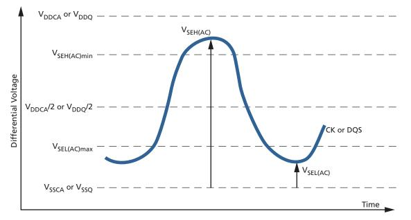
Note that while CA and DQ signal requirements are referenced to  $V_{REF}$ , the single-ended components of differential signals also have a requirement with respect to  $V_{DDO}/2$  for DQS, and  $V_{DDCA}/2$  for CK.
