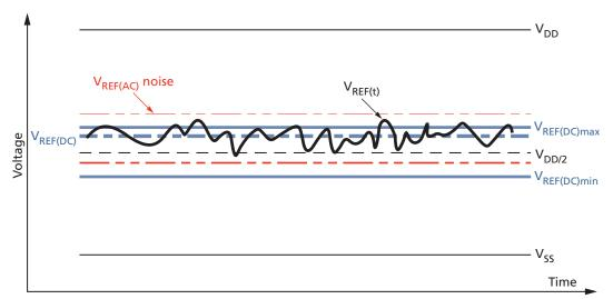
The voltage levels for setup and hold time measurements  $V_{IH(AC)}, V_{IH(DC)}, V_{IL(AC)}$ , and  $V_{IL(DC)}$  are dependent on  $V_{REF}$ .
