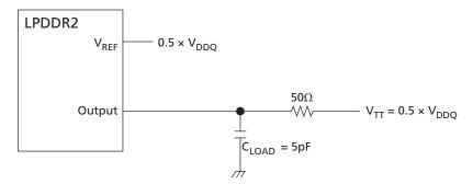
Note: 1. All output timing parameter values (<sup>t</sup>DQSCK, <sup>t</sup>DQSQ, <sup>t</sup>QHS, <sup>t</sup>HZ, <sup>t</sup>RPRE etc.) are reported with respect to this reference load. This reference load is also used to report slew rate.
