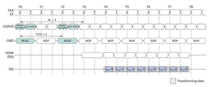
Figure 21: Seamless Burst READ – RL = 3, BL = 4, <sup>t</sup>CCD = 2
