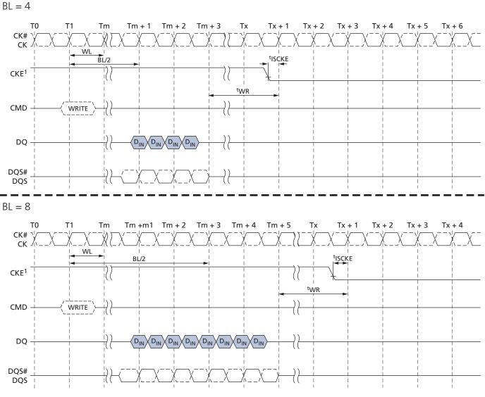
Note: 1. CKE can be registered LOW at (WL + 1 + BL/2 + RU(<sup>t</sup>WR/<sup>t</sup>CK)) clock cycles after the clock on which the WRITE command is registered.
