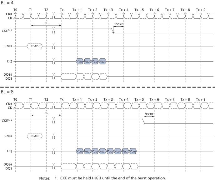
CKE can be registered LOW at (RL + RU(<sup>t</sup>DQSCK(MAX)/<sup>t</sup>CK) + BL/2 + 1) clock cycles after the clock on which the READ command is registered.
