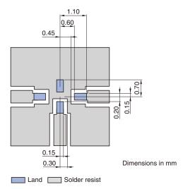
Line width should be designed to match  $50\Omega$  characteristic impedance, depending on PCB material and thickness.
