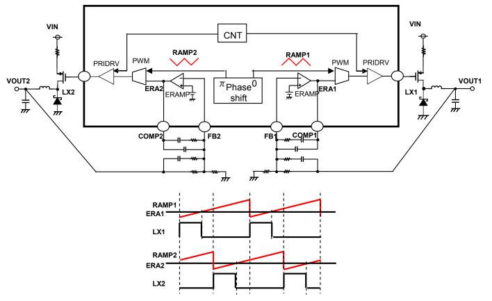
図: Channel-to-channel phase reversal function Block diagram and timing chart
