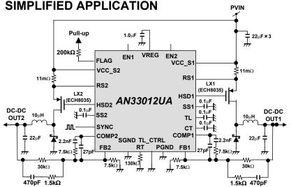
Notes) This application circuit is an example. The operation of mass production set is not guaranteed. You should perform enough evaluation and verification on the design of mass production set. You are fully responsible for the incorporation of the above application circuit and information in the design of your equipment.
