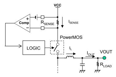
Figure: Over-Current Protection circuit block diagram
