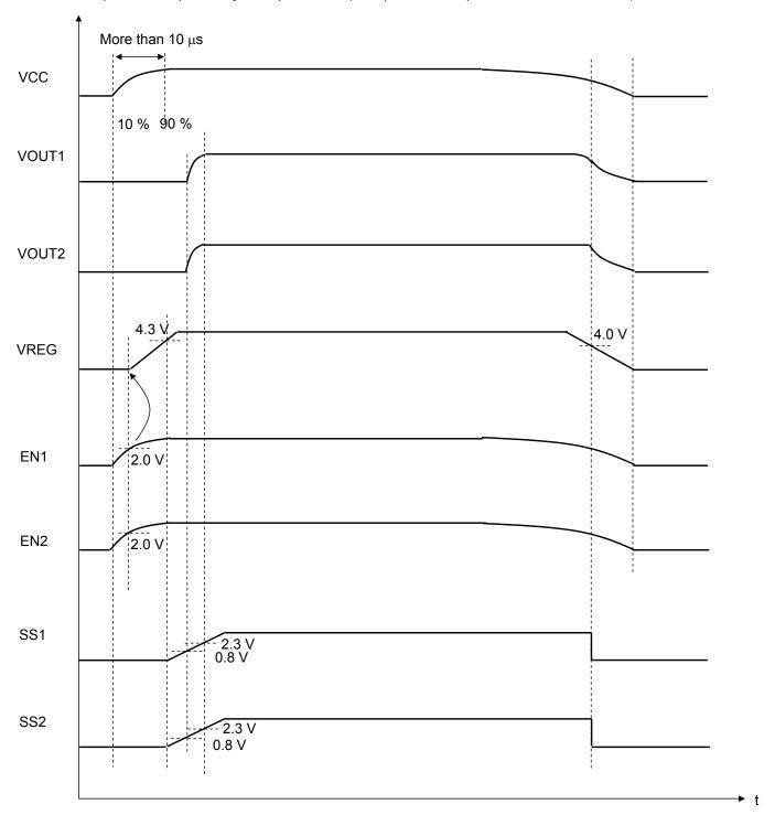
Figure: Power ON/OFF sequence by VCC/EN1/EN2
