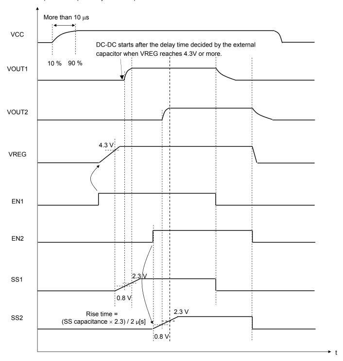
Figure: Power ON/OFF sequence by EN1/EN2
