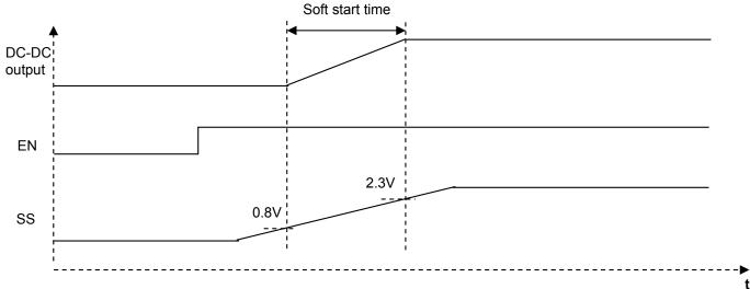
Figure: Soft start operation timing chart
