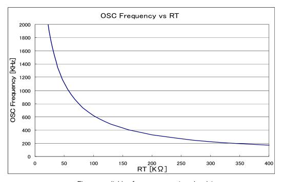
Figure: switching frequency vs external resistance
