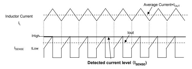
Figure: Method of detection of Over-Current Protection function
