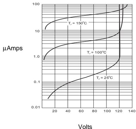
Instantaneous Reverse Leakage Current - MicroAmperes versus
