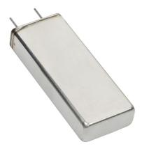
With a profile of 1.0" by 0.5" type MLSG Slimpack capacitors fit into the tightest of spaces and meets a DC test of 5000 hrs at rated voltage, 125 °C. MLSG Slimpack is a perfect fit for military and aerospace applications requiring a low profile, rugged design and long-life. Specify type HRMLSG for high reliability burn-in.
