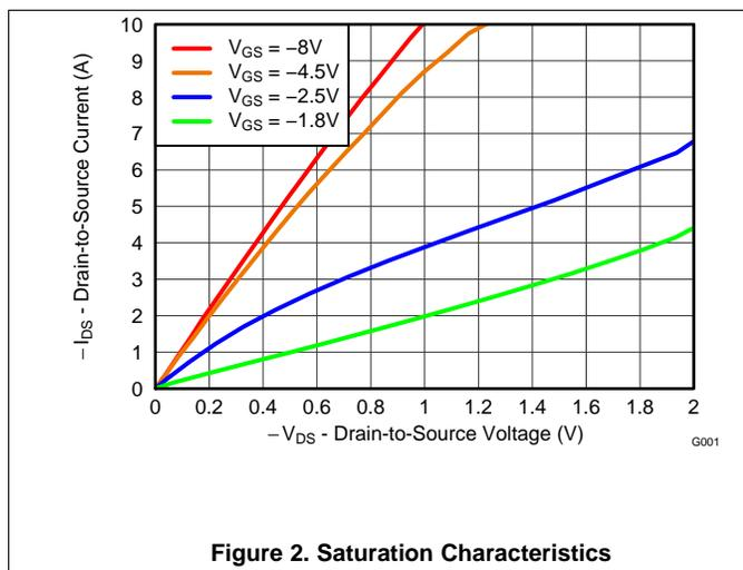
Figure 2. Saturation Characteristics
