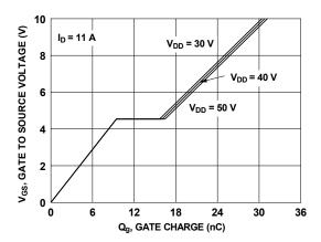
Figure 7. Gate Charge Characteristics
