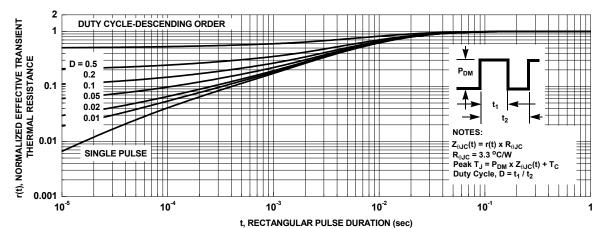
Figure 13. Junction-to-Case Transient Thermal Response Curve
