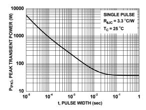
Figure 12. Single Pulse Maximum Power Dissipation
