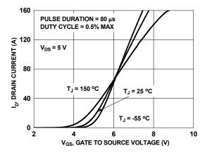
Figure 5. Transfer Characteristics
