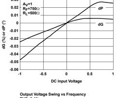
Differential Gain/Phase vs DC Input Voltage at 3.58MHz
