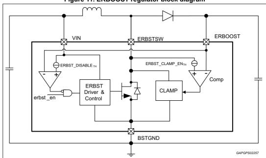
Figure 11. ERBOOST regulator block diagram
