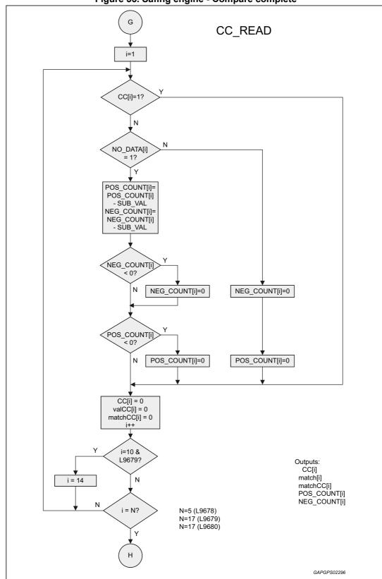
Figure 55. Safing engine - Compare complete
