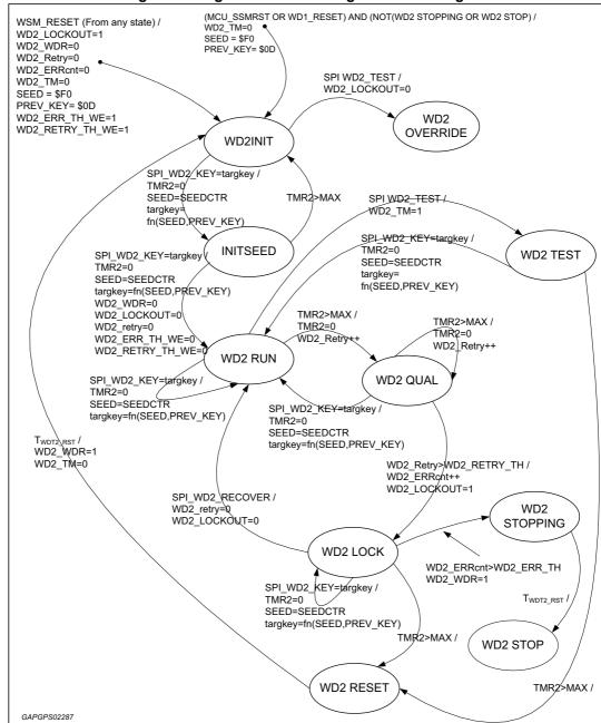
Figure 46. Algorithmic watchdog timer flow diagram
