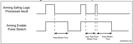
Figure 61. Pulse stretch timer example
