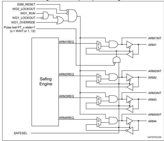
Figure 60. ARMx input/output control logic
