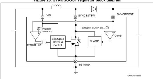
Figure 20. SYNCBOOST regulator block diagram
