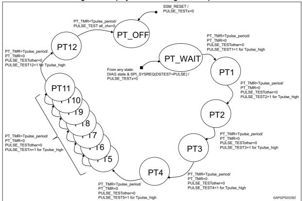
Figure 35. Deployment timer diagnostic sequence
