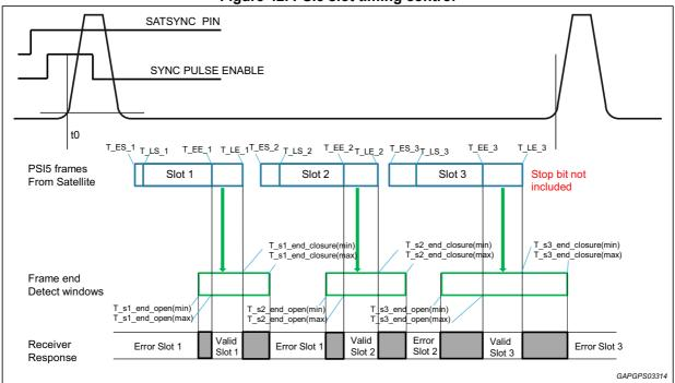
Figure 42. PSI5 slot timing control
