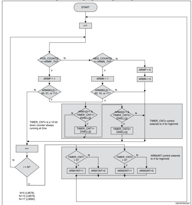
Figure 58. Safing engine arming flow diagram
