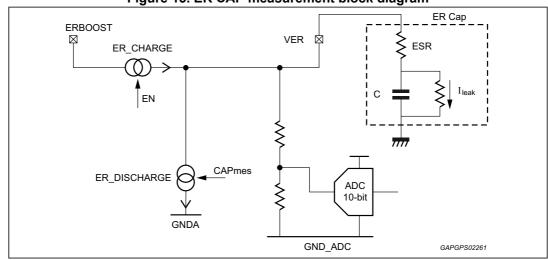
Figure 15. ER CAP measurement block diagram
