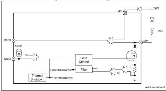
Figure 67. ISO9141 block diagram
