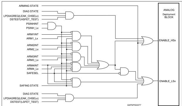
Figure 28. Deployment driver control logic - Enable signal
