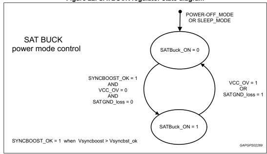
Figure 22. SATBUCK regulator state diagram
