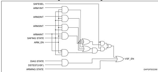
Figure 24. VSF control logic
