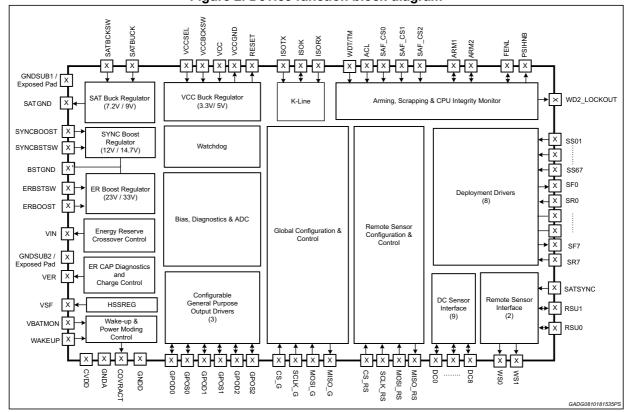
Figure 2. Device function block diagram
