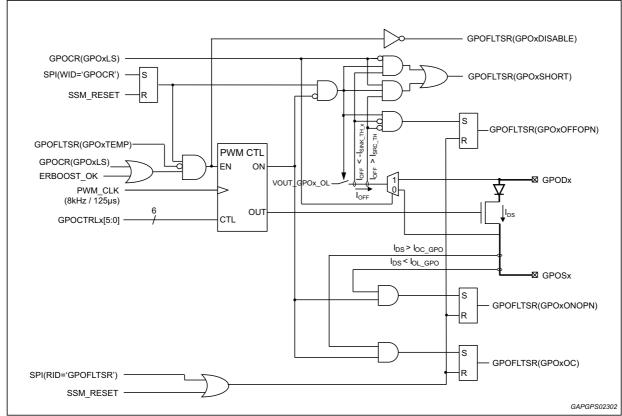
Figure 65. GPO driver and diagnostic block diagram
