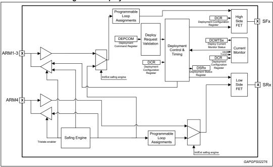
Figure 27. Deployment driver control blocks
