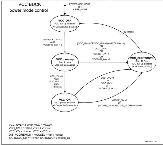
Figure 23. VCC regulator state diagram
