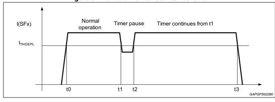
Figure 32. Current monitor counter behavior
