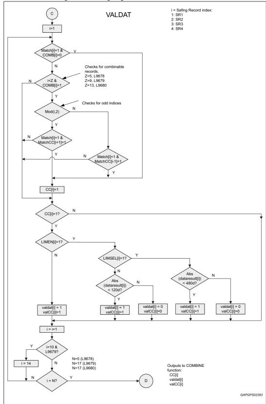
Figure 52. Safing engine - Validate data flow chart
