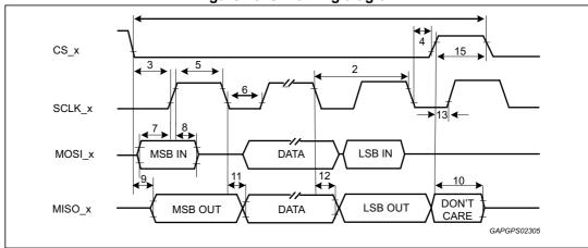
Figure 70. SPI timing diagram
