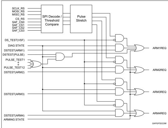
Figure 59. Safing engine diagnostic logic
