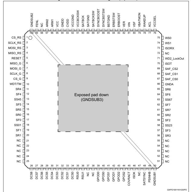
Figure 1. Pin connection diagram (top view)
