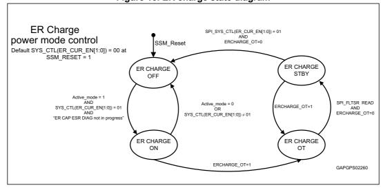
Figure 13. ER charge state diagram
