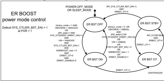
Figure 12. ERBOOST regulator state diagram
