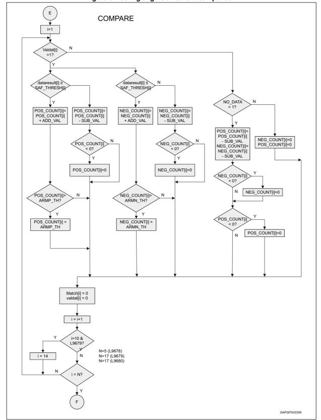
Figure 54. Safing engine threshold comparison
