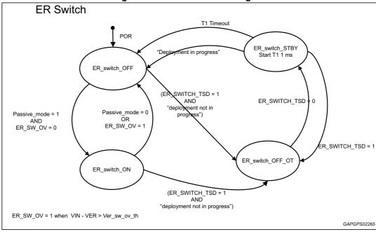
Figure 19. ER switch state diagram
