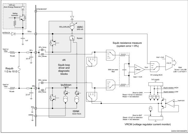
Figure 33. Deployment loop diagnostics
