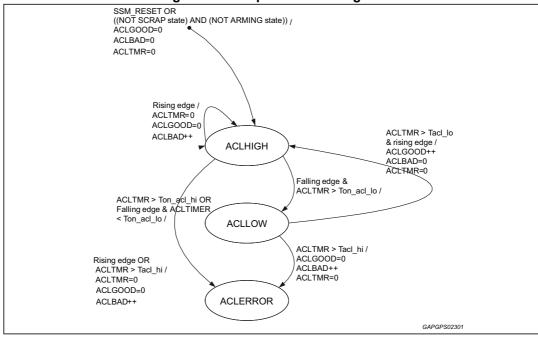
A specific waveform needs to be present on ACL input in order to instruct L9679P to arm all deployment loops. L9679P is designed to support the Additional Communication Line (ACL) aspect of the ISO-26021 standard, which requires an independent hardwired signal (ACL) to implement the scrapping feature. The disposal signal may come from either the vehicle's service connector, or the systems main microcontroller, depending on the end customer's requirements.
