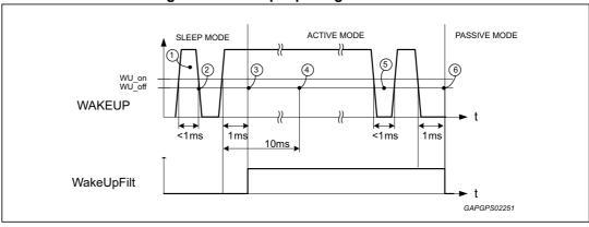
Figure 5. Wake-up input signal behaviour
