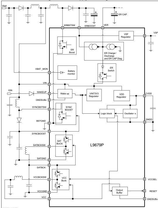
Figure 3. Power supply block diagram
