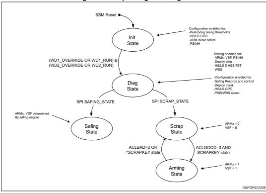
Figure 10. IC operating state diagram
