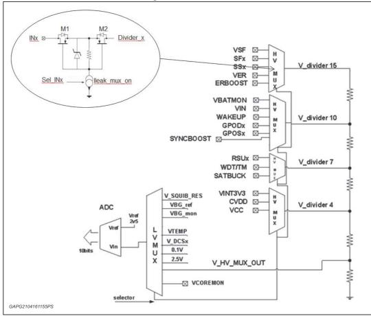
Figure 68. ADC MUX
