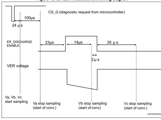
Figure 18. ER ESR measurement timing diagram
