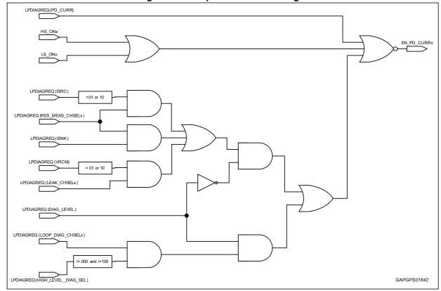
Figure 34. SRx pull-down enable logic
