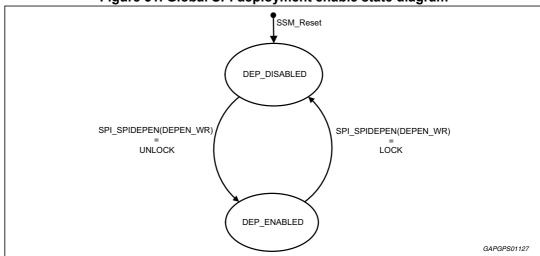
Figure 31. Global SPI deployment enable state diagram
