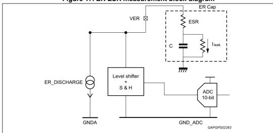
Figure 17. ER ESR measurement block diagram
