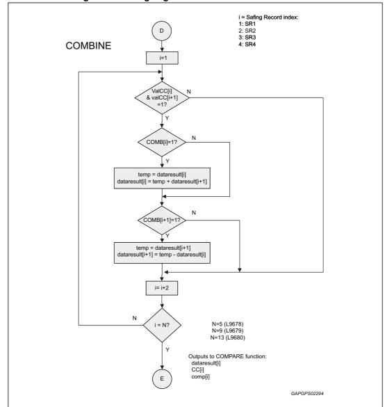
Figure 53. Safing engine - Combine function flow chart
