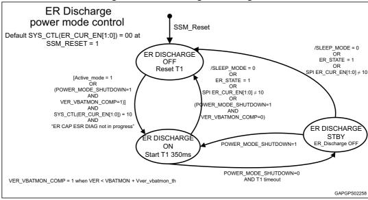
Figure 14. ER discharge state diagram
