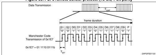
Figure 39. PSI-5 remote sensor protocol (10-bit, 1-bit parity
