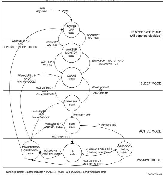
Figure 4. Power control state flow diagram
