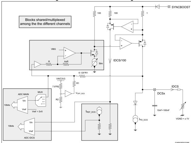
Figure 47. DC sensor interface block diagram
