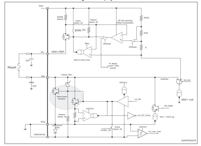
Figure 30. Deployment driver block
