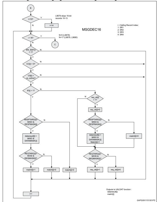
Figure 51. Safing engine - 16-bit Message decoding flow chart
