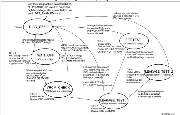
Figure 36. High level loop diagnostic flow1
