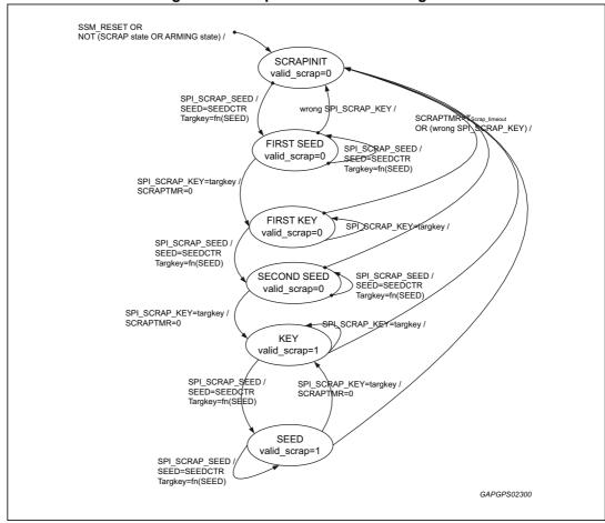
Figure 62. Scrap SEED-KEY state diagram
