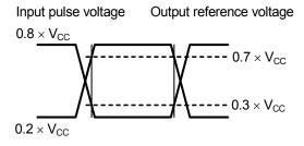
Figure 4 I/O Waveform during AC Measurement
