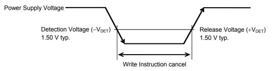
Figure 19 Operation during Low Power Supply Voltage
