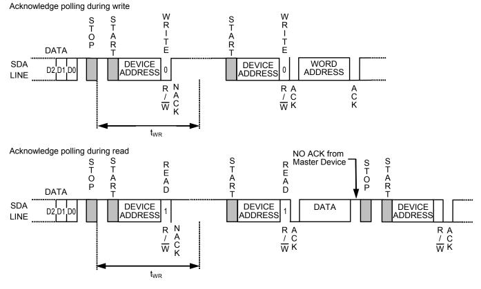
**Remark** Users are able to input word address and data after ACK output in acknowledge polling during write. Users are able to read data after ACK output in acknowledge polling during read. However, after that users input the write instruction, a start condition may not be input during data output. Input a stop condition and the next instruction after data output and ACK output.
