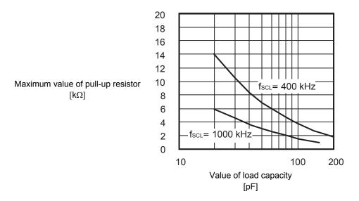
Figure 7 Output Load
