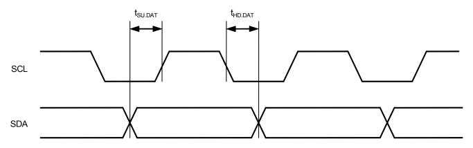
Figure 9 Data Transmission Timing
