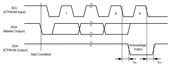
Figure 10 Acknowledge Output Timing
