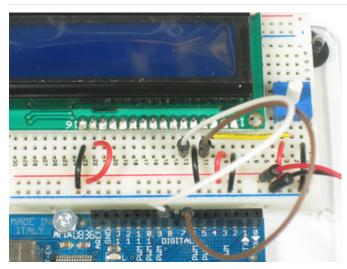
Next is the **EN** pin #6, we'll use a white wire to connect it to Arduino digital #8.
