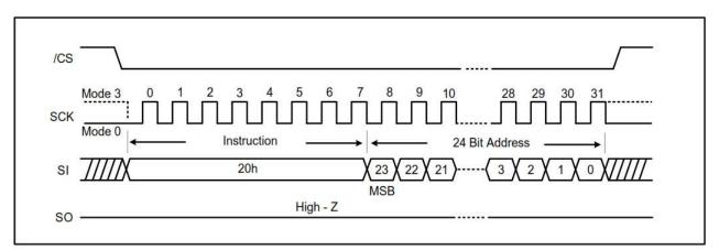
Figure 7-26. Block Erase Instruction (SPI Mode)
