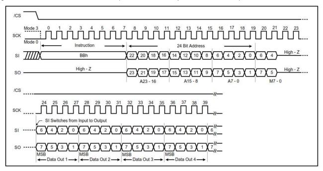
Figure 7-17. Fast Read Dual I/O Instruction (previous M7-0= Axh)
