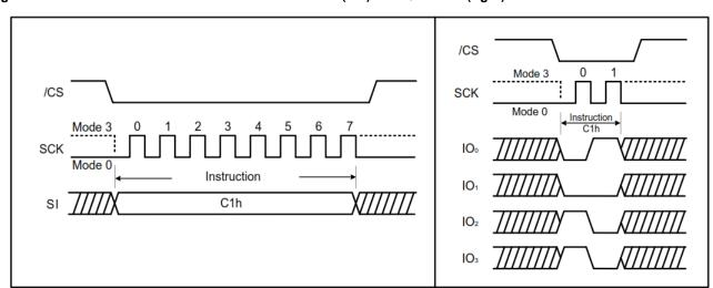
Figure 7-60. Exit Secured OTP Instruction for SPI Mode (left) and QPI Mode (right)
