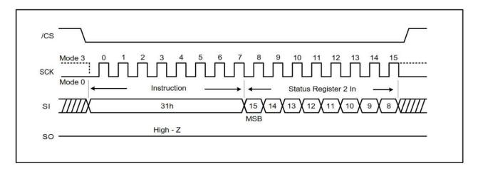
Figure 7-9. Write Status Register-2 Instruction (QPI Mode)
