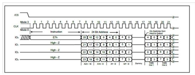
Figure 7-51. Word Read Quad I/O Instruction (Previous instruction set M7-0= Axh, SPI Mode)
