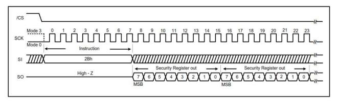
Figure 7-62. Read Security Register Instruction (QPI Mode)
