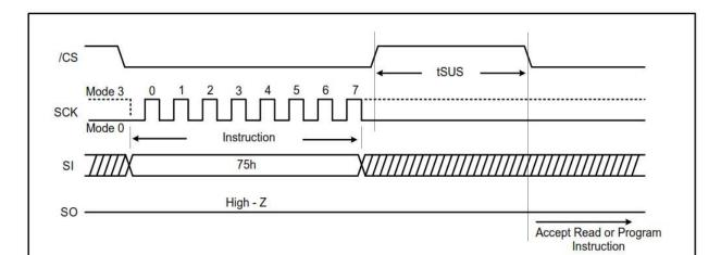
Figure 7-33. Erase Suspend Instruction (SPI Mode)
