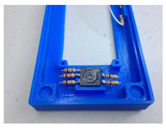
Push the joystick into the square opening. It should be a tight fit. If not, put a little bit of super glue along the seam to fix the joytick in place.
