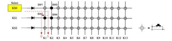
So instead of writing code for debouncing the buttons on the Pro Trinket, we can ask the HT16K33 over I2C about the state of all buttons once every 20ms (50Hz). That's exactly what we are doing in this tutorial!
