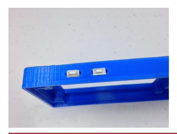
Be careful when soldering inside the enclosure. Your soldering iron will deform the PLA plastic if they come in contact with each other (see the burn mark in the picture below.)
