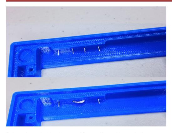
On the inside, you should be able to see all four pins of the pushbuttons. Bend the inner two and join them together
