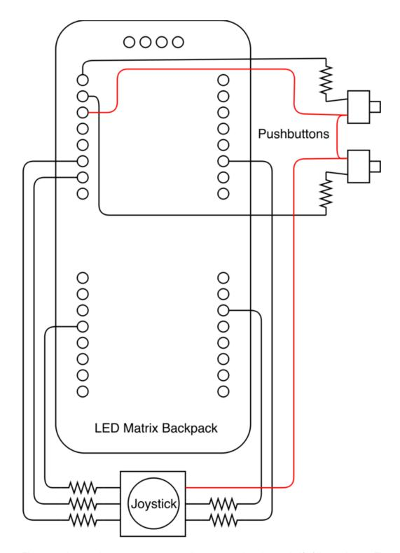
The second circuit diagram contains everything mounted on the top half of the enclosure. This is a view from the inside of the enclosure, which means that both the LED Matrix Backpack and the joystick are facing away from us. If it seems confusing, the assembly guide on the next page will definitely help you understand better. All seven resistors shown in this circuit diagram have a value of  $10k\Omega$ .
