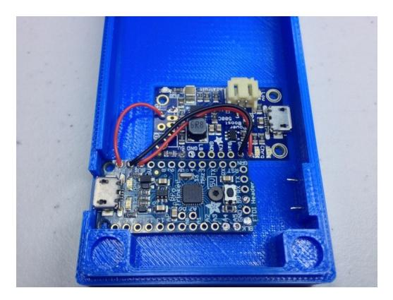
Use three short wires to connect the power lines between the PowerBoost and the Pro Trinket.
