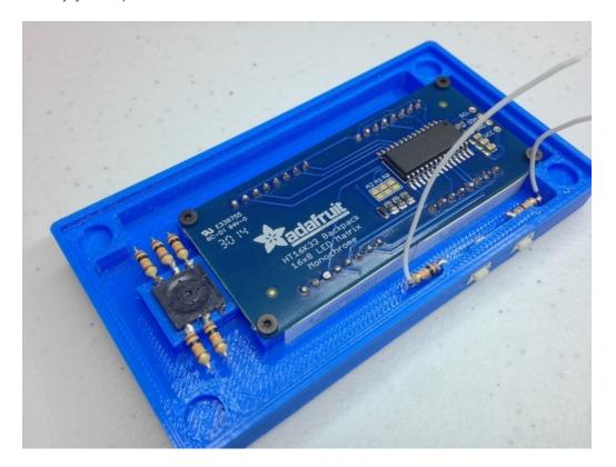
Now push the LED matrix backpack into the largest opening, and use four M2 screws to secure it in place. Make sure that the I2C pins (VCC, GND, SCL, SDA) are near the top of the device.
