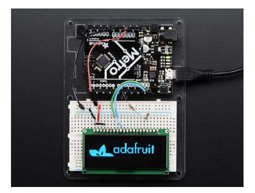
Don't forget you have to set the display to I2C mode, see the Assembly step on how to do that!
