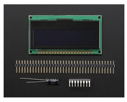
Each order comes with one assembled OLED module with a nice bezel and 4 mounting holes. The display is 3V logic &
