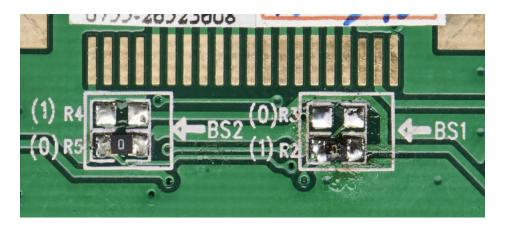
(If you solder and re-solder the resistors 10 times like I did while figuring out all the setting and wiring, you'll get a kinda messy/fluxy look like the above! In that case you can clean up with some IPA wipes. Or just revel in your punk soldering job)
