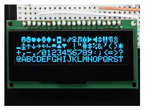
The driver chip, SSD1305 can communicate in three ways: 8-bit, I2C or SPI. Personally we think SPI is the way to go,
