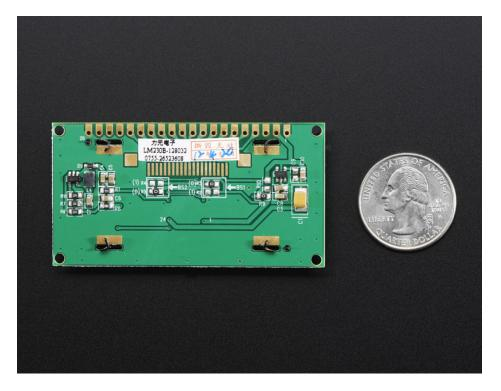
Getting started is easy! We have a detailed tutorial and example code in the form of an Arduino library for text and graphics. (https://adafru.it/j6a) You'll need a microcontroller with more than 512 bytes of RAM since the display must be buffered. The library can print text, bitmaps, pixels, rectangles, circles and lines. It uses 512 bytes of RAM since it needs to buffer the entire display but its very fast! The code is simple to adapt to any other microcontroller.
