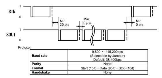
Note: Output data is transferred collectively from a VFD module, so a receiving buffer may be required on a host system to prevent data loss.
