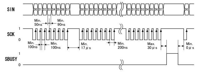
Note: Monitoring the serial busy line (SBUSY) is strongly recommended, because it prevents data loss and minimizes a waiting time to write next data. Please write data when SBUSY = 0.
