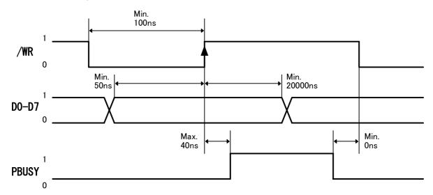
Note: Monitoring the parallel busy line (PBUSY) is strongly recommended, because it prevents data loss and minimizes a waiting time to write next data. Please write data when PBUSY = 0.
