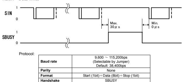
Note: Monitoring the serial busy line (SBUSY) is strongly recommended, because it prevents data loss and minimizes a waiting time to write next data. Please write data when SBUSY = 0.
