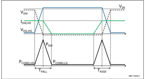
Figure 9. Switching losses
