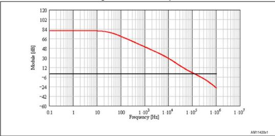
Figure 7. Module bode plot
