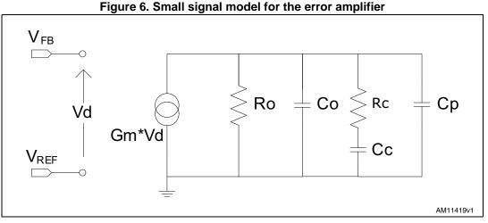
$R_C$  and  $C_C$  introduce a pole and a zero in the open loop gain.  $C_P$  does not significantly affect system stability and can be neglected.
