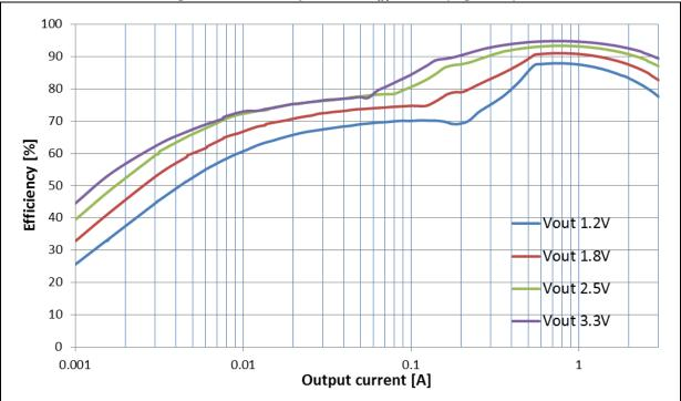
Figure 21. Efficiency curves: V<sub>IN</sub> = 5.0 V (log scale)
