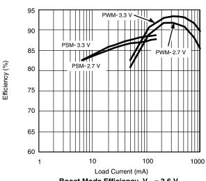
Boost Mode Efficiency,  $V_0 = 3.6 \text{ V}$
