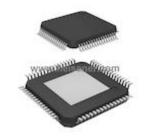
Part NumberLAN9252T/PTManufacturerMicrochip TechnologyCategoryIntegrated Circuits (ICs)<br/>Interface - ControllersDescriptionIC ETHERCAT CTLR 10/100 64TQFPPackage64-TQFP Exposed Pad<br/>For the pricing/inventory/lead time, please contact<br/>us<br/>Website: https://www.heisener.com<br/>E-mail: salesdept@heisener.com
