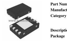
Part NumberLTC6930HDCB-4.19#TRMPBFManufacturerLinear TechnologyCategoryIntegrated Circuits (ICs)<br/>Clock/Timing - Programmable Timers and<br/>OscillatorsDescriptionIC OSC SILICON 4.194304MHZ 8-DFNPackage8-WFDFN Exposed Pad<br/>For the pricing/inventory/lead time, please contact<br/>us<br/>Website: https://www.heisener.com<br/>E-mail: salesdept@heisener.com
